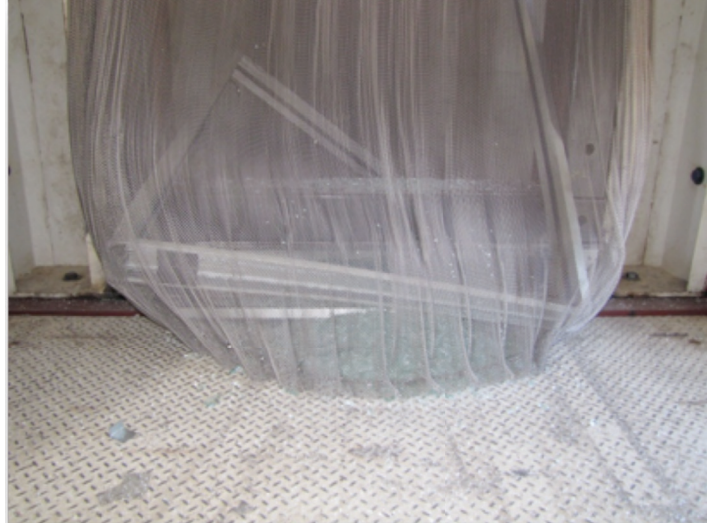
Baker Shock Tube Blast Test 1/4"-19ga. Steel
